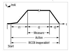
The test instrument generates a DC residual current which saturates the magnetic circuit of the RCCB. The PROFITEST®C superimposes a measuring current which demonstrates only half-waves of like polarity. The RCCB cannot detect
