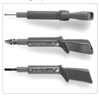
Three self-retaining, contact protected test probes for the connection of measurement cables with 4 mm banana plugs, or with contact protected plugs for sockets with an opening of 3.5 mm to 12 mm, e.g. CEE and Perilex sockets etc. The test probes also fit the square PE jacks on Perilex sockets. Maximum allowable operating voltage: 600 V per IEC 61010.
